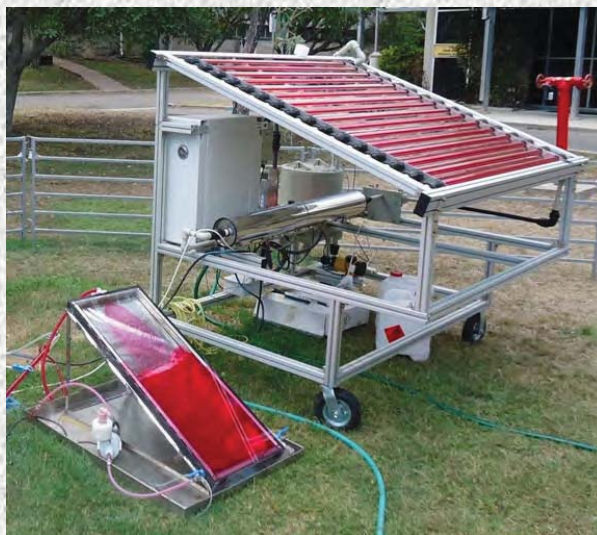
Figure 1: Solar reactors at James Cook University. The red color of the photosensitizer rose Bengal can be clearly seen.
